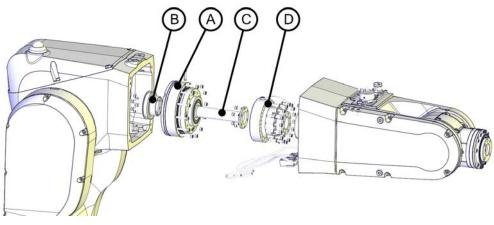
1.10.5 Spare parts - axis-5 and axis-6 drive unit
